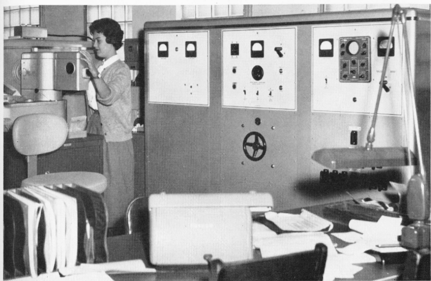
Nancy Lawson is placing a sample on the electrode stand of the Quantometer. After she turns the switch, an automatically controlled spark will pass between the surface of the sample and the carbon electrode.
